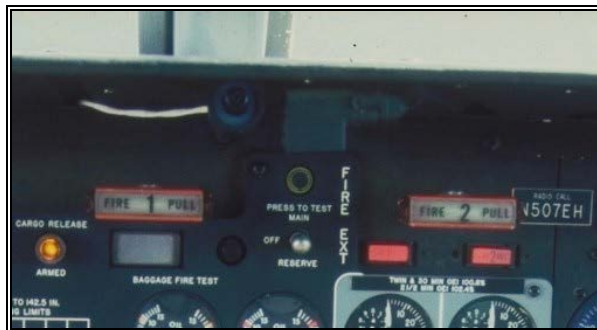
Figure 13-20b Fire Pull Handles
